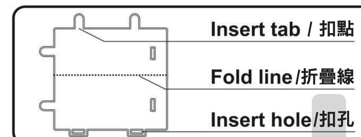
Identify the insert tab, fold line and the insert hole.
