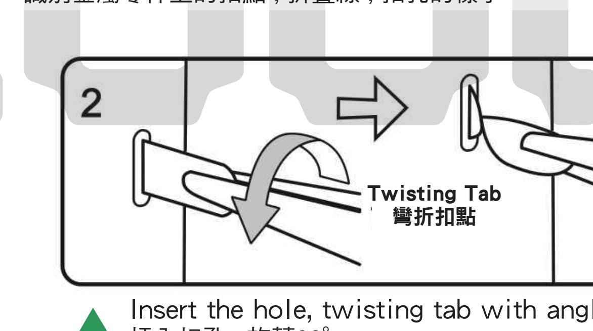
Insert the hole, twisting tab with angle 90°
