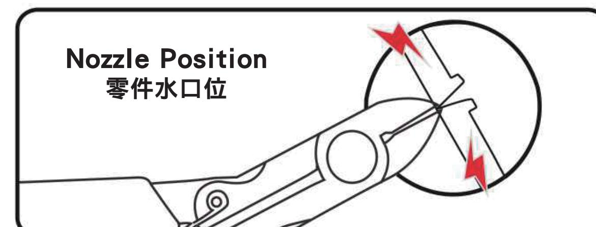
Please use the clipper to cut the nozzle position and remove the parts.
