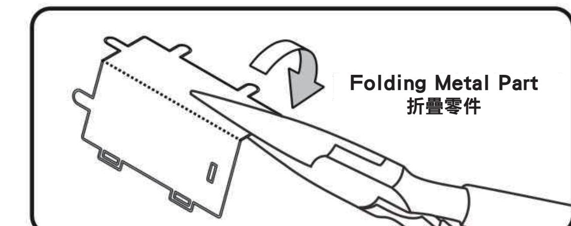
Please use the Needle nose pliers to fold the cutting parts into models.
