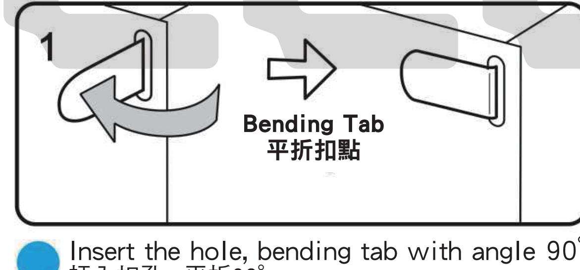
Insert the hole, bending tab with angle 90°
