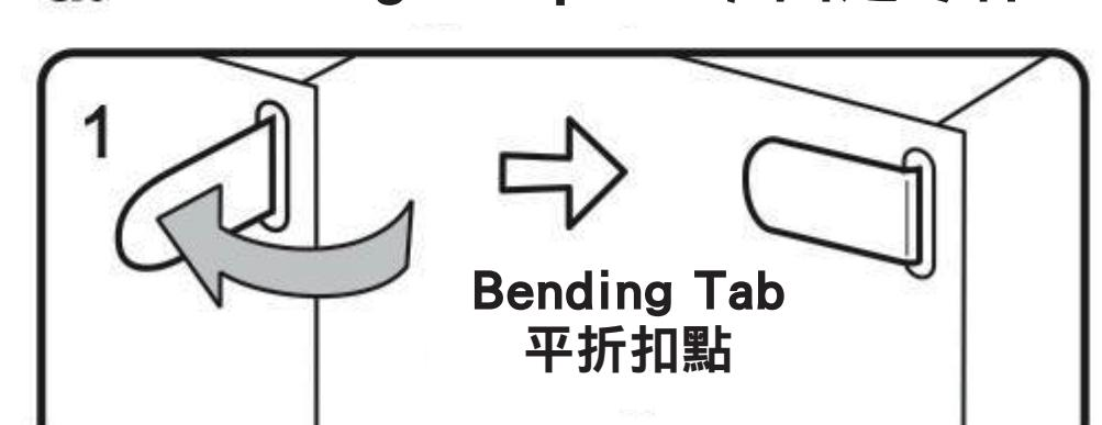
Insert the hole, bending tab with angle 90°
