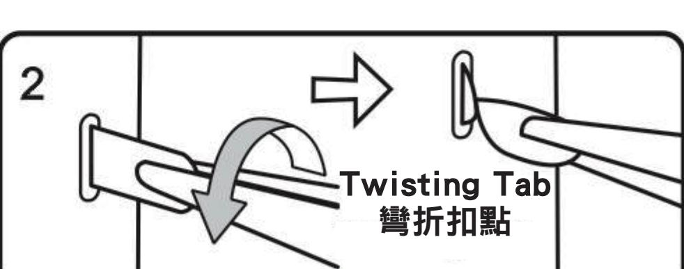
Insert the hole, twisting tab with angle 90°
